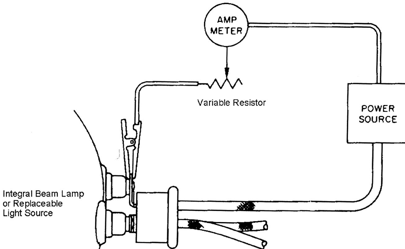
Figure 11 - Connector Test
