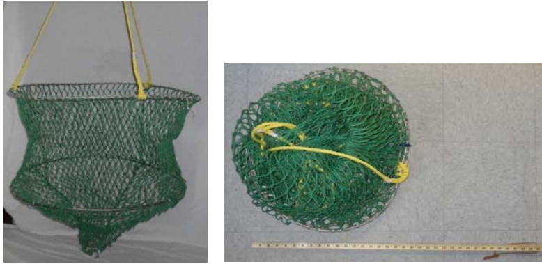
Figure 1.2.1.1. Example of a collapsible hoop net open and ready to be stored when folded. Photo credit: NMFS-SEFSC
