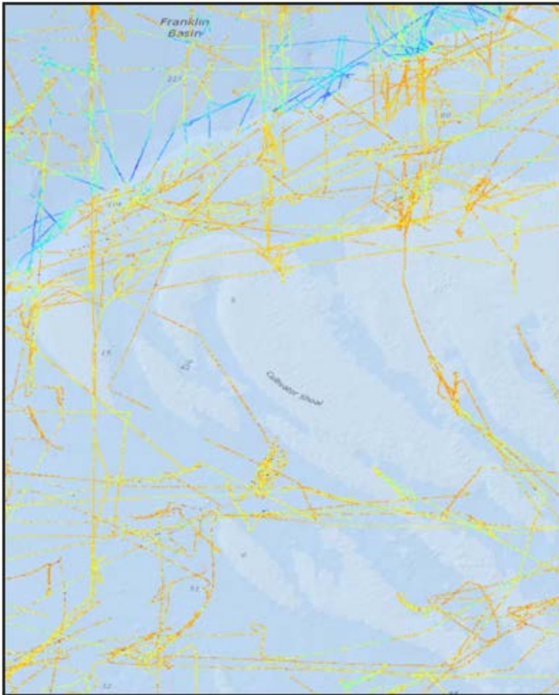
Figure 260: Hardness on Cultivator shoals, Georges Bank as estimated from multifrequency acoustic data collected along the tracks of NOAA ships. The data are displayed on a blue to red scale where redder colors are harder and bluer colors are less hard.
