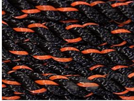
Figure 2.10.2. Example of a color tracer line (orange) woven along the entire length of a black trap line. In the image, the trap line is coiled.
