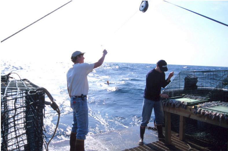
The horizontal long line consisted of 1676 m of 3.2 mm galvanized cable deployed from a longline reel. The groundline was 1219 m and the remaining 457 m was buoyed to the surface.
