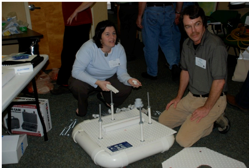
Angela Bliss from University of Georgia and Jim Nelson from Skidaway Institute of Oceanography assemble a BOB, a Basic Observation Buoy designed to teach students from kindergarten through graduate school about observing technologies. Image Credit: Lundie Spence, COSEE-SE
