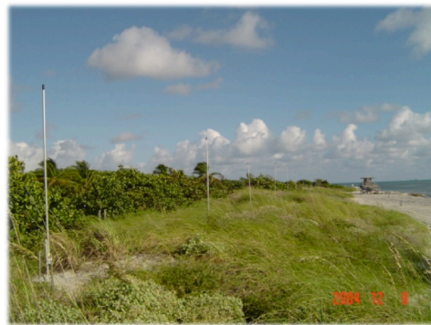
The medium and long-range Wellen Radars (WERA) deployed along the Florida Straits and the South Atlantic Bight have a spatial resolution of 1.2 to 3 km and sample at time scales of minutes. Photo: Nick Shay/WERA System/Crandon Park
