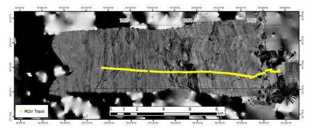
*Figure 6-7. Priority Area 3 multibeam backscatter data. The yellow line illustrates the primary ROV transect. The northeastern transect, which lay chiefly beyond the area surveyed by multibeam, is omitted from this image (see Figure 6-6).*
