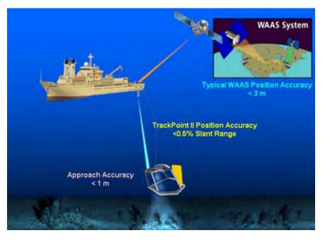
Figure 6-10. Television Observed Nautical Grappling System (TONGS).
