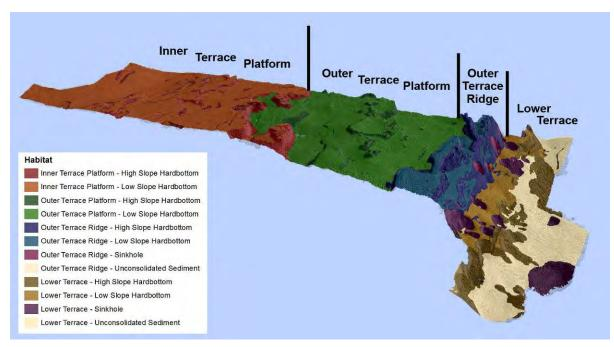
Figure 6-9. Three-dimensional rendering multibeam topography overlain by the benthic habitats illustrating the four major geomorphological features of Priority Area 3.
