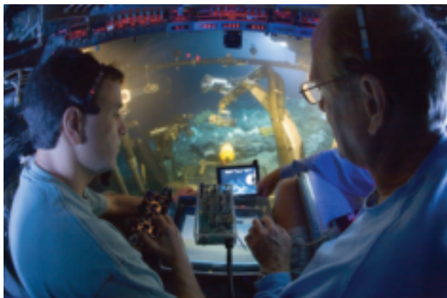
Deep coral researcher John Reed and pilot Phil Santos dive the Johnson-Sea-Link submersible on a deepwater reef in the Straits of Florida. A manipulator arm is used to reach out and collect specimens of corals and sponges for research.
