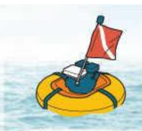
The compressor Can be onboard a boat or on a floating tube.
