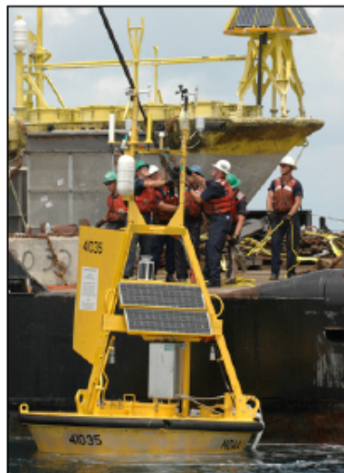
The USCG ELM deploys a UNCW/US Marine Corps weather and oceanographic buoy 5 miles offshore of the Camp Lejeune Marine Corps Base. The buoy provides valuable data for boaters and mariners and plays a significant role in military training and Base operations. Photo: UNCW/Jamie Moncrief
