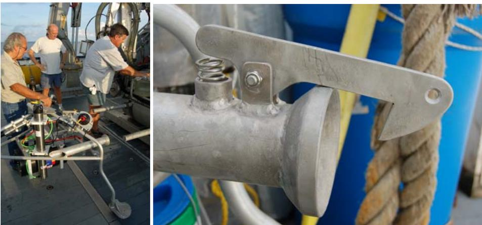
**Fig. 1:** Photographs showing the microlander frame about to be lifted onto the poles projecting from the bow of the JSL submersible and the hook mechanism that locked the frame to the submersible.
