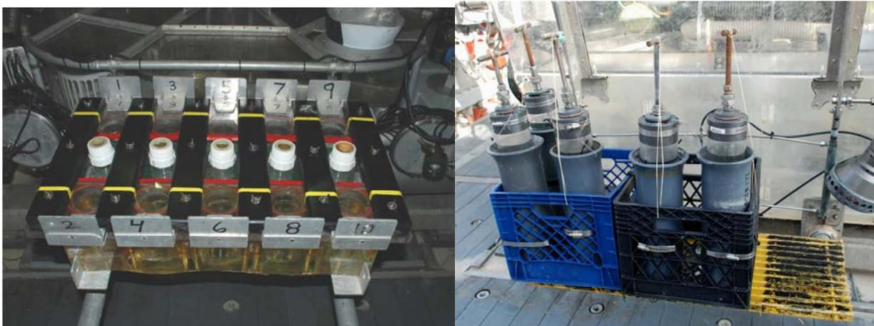
Figure 4. Kellogg sampler (left) for collecting isolated coral samples and push tube cores (right) used for sediment collections. Both are mounted to the bow of the JSL submersible.
