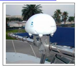
"The CLS Thorium LRIT terminal is an automatic satellite tracking system based on the Iridium network and developed in compliance with the international IMO regulations. Easy to install, secure and robust, this transceiver perfectly suits all types of vessels. Thorium is compatible whatever the ship's location, including A4.
