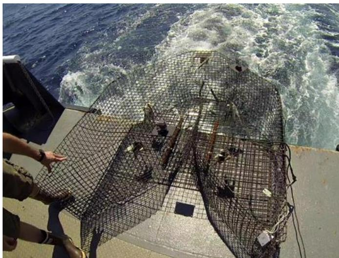
**Figure 4.** Chevron trap baited with Menhaden, ready for deployment. Note, iron sashes were used to weigh the trap down, thus promoting the proper orientation, and stabilizing the trap, on the bottom.
