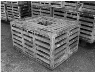
Figure 2.3 Example of a Commercial Spiny Lobster Trap
