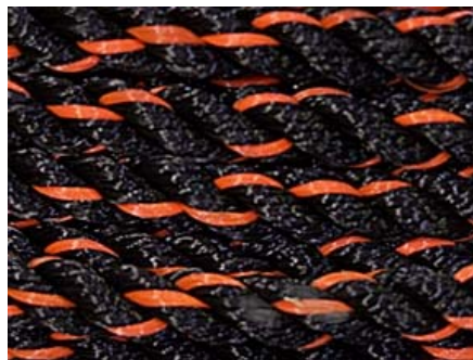
Figure 2.10.1. Example of a color tracer line (orange) woven along the entire length of a black trap line. In the image, the trap line is coiled.
