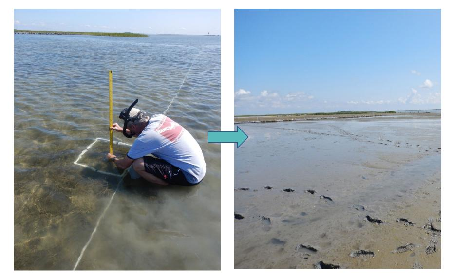
The coir log structure was not effective at containing the placed sediments; the 2 acre SAV bed was buried by ~30 cm of sediment – but keeping the island in place serves to protect the much larger (~150 acre) SAV bed to the south
