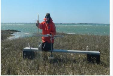
Changes in sediment surface elevation translate directly into differences in pin length above the SET arm There are 132 SETs installed across the NC coast, these devices have associated data records of between 5 and 30 years
