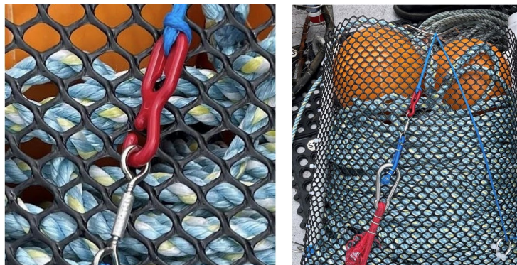
Figure 13. Longsoaker GTR system installed on Terhune Bag
