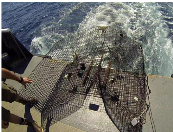
Figure 3. CHV equipped with cameras (chevron-video trap, CVT) and baited with menhaden, ready for deployment. Note, iron sashes were used to weigh the trap down, thus promoting the proper orientation, and stabilizing the trap, on the bottom.
