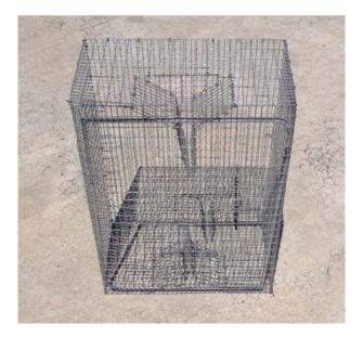
Height: 10.5" Width: 18" Length: 24" Galvanized wire mesh, biodegradable panel and concrete ballast to be added. Dual funnel: One at each end of trap not to exceed 7" in length x 4" width 4. South Atlantic Commercial Sea Bass Trap (As defined in CFR 622.189)
