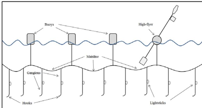
Figure 3.2 Typical U.S. Pelagic Longline Gear
