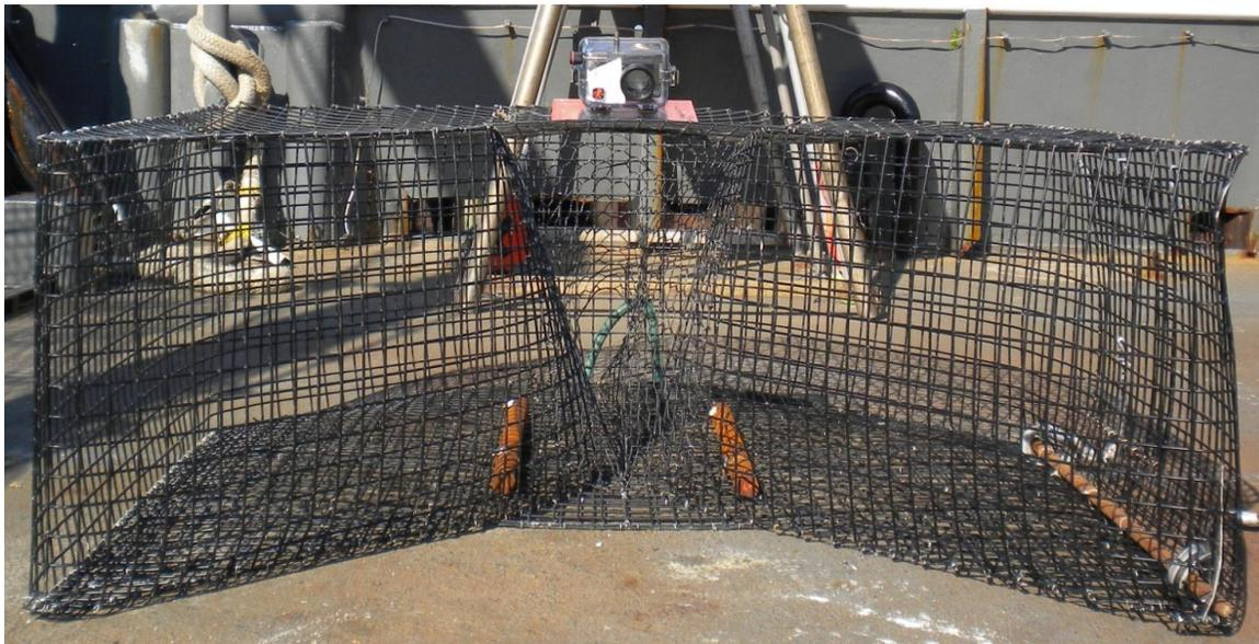
**Figure 2.** Chevron trap with camera mounted above trap opening.
