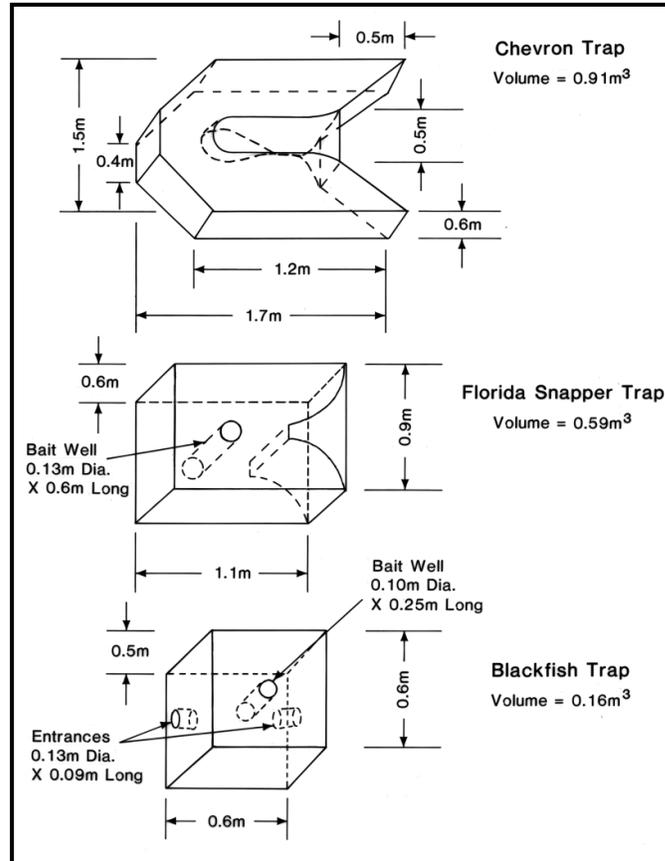
**Figure 1.** Diagrams of the three most frequently used traps by MARMAP (From Collins, 1990).
